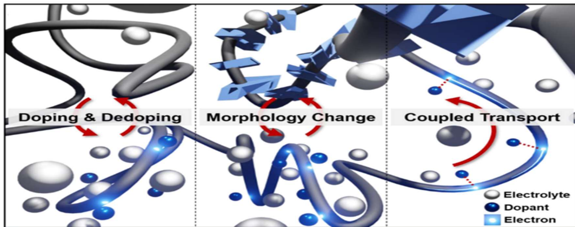
Figure 3. Schematic diagram of three central process in OMIECs. The first process (left) is doping and dedoping; second (center) is the morphology changes upon ion penetration; last (right) is the ion-coupled electron transport 13 .
