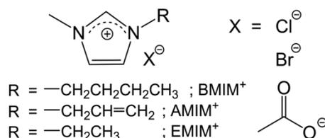
**Figure 2.** Common ionic liquids used to dissolve cellulose  $I\beta$  bonds. Figure from Ref 2.
