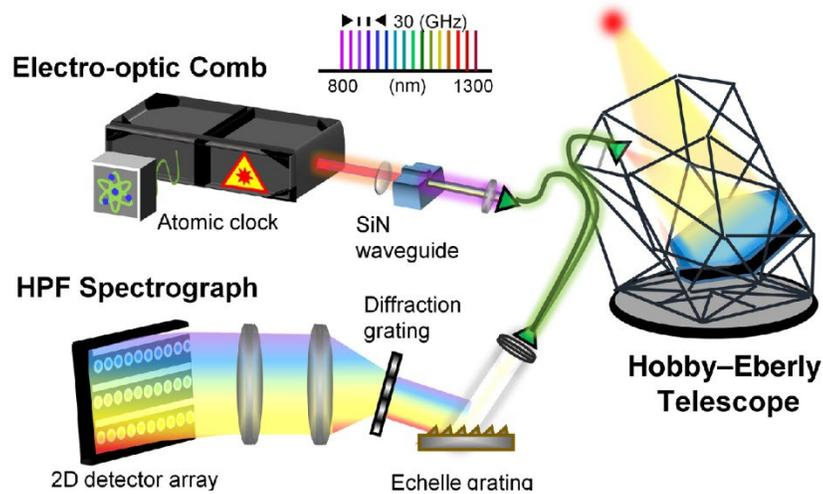
**Figure 2.** The instrumentation for precision infrared radial velocity spectroscopy is shown from Ref 1. Starlight was collected by the Hobby-Eberly telescope and directed to an optical fiber. To generate a frequency comb with teeth spaced 30 GHz, lasers, electro-optics, and nanophotonics were used, and the comb was stabilized using an atomic clock. Both the starlight and frequency comb light were coupled to the highly stabilized Habitable Zone Planet Finder (HPF) spectrograph.
