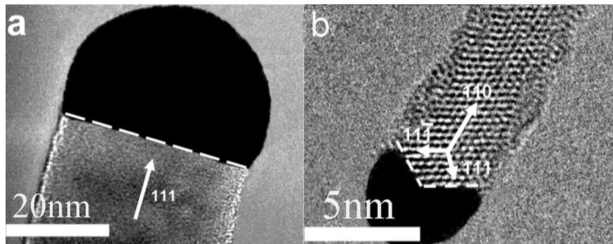
**Figure 1:** TEM image of the catalyst alloy/NW interface of a Si NW with a  $\langle 111 \rangle$  growth axis (part a) and  $\langle 110 \rangle$  growth axis (part b).
