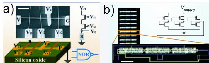
**Figure 3:** a) Schematic of logic NOR gate constructed from 1 by 3 crossed NW junction array. b) Optical images and circuit diagram of nanowire ring oscillators. Scale bar: 100 $\mu$ m.
