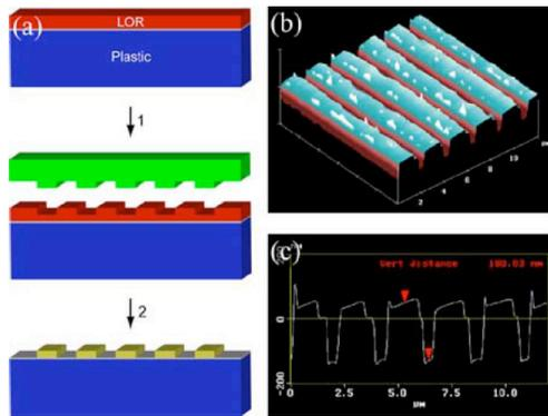
**Fig. 2.** a) Schematic of the NIL process on plastic. (b) and (c) AFM topographical and line-scan images of the imprinted features, respectively.
