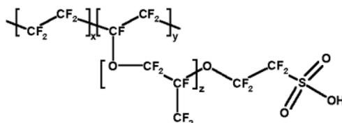
**Figure 2:** General chemical structure of Nafion ionomers.
