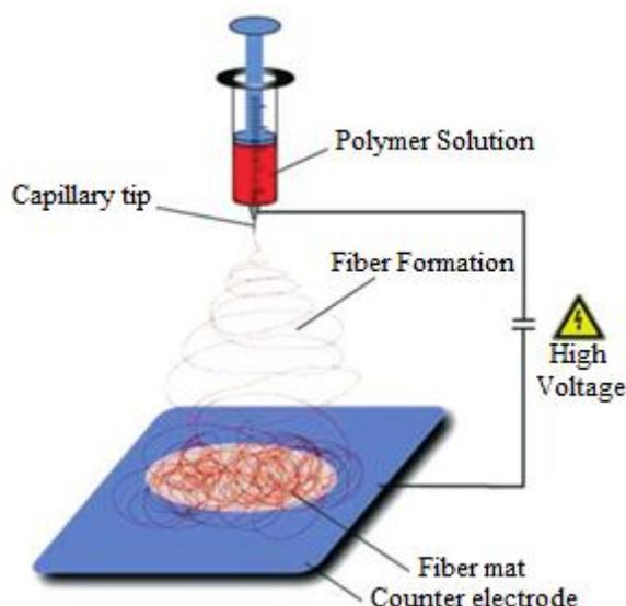
**Figure 1:** Cartoon schematic of an electrospinning experiment.<sup>1</sup>
