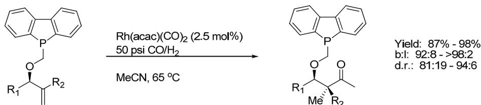
**Scheme 3. Directed Diastereoselective Branched Hydroformylation of Allylic Alcohols.**
