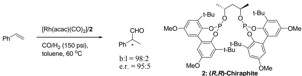
**Scheme 4. Asymmetric Hydroformylation of Styrene with Rh-Chiraphite.**
