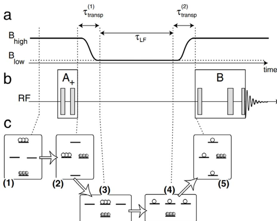
FIG 1. (a) Magnetic field scheme used in generating long-lived singlet state; (b) pulse sequence used to generate long-lived singlet state; (c) a schematic depiction of the two-spin system during the period of experiment.
