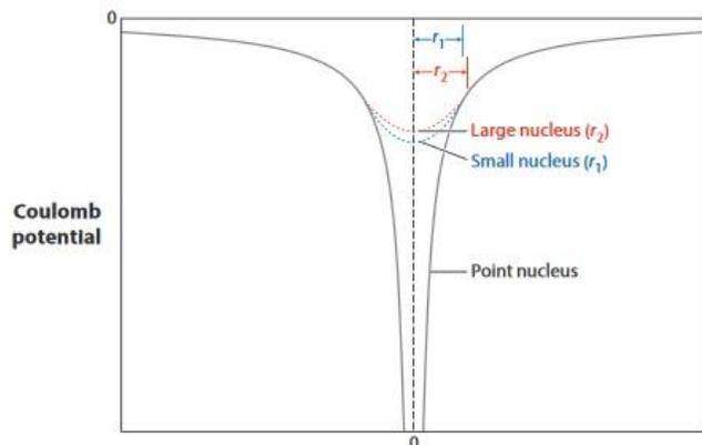
Figure 1. Electrostatic potential binding of an electron to a nucleus. It is higher for a larger nucleus than a smaller one<sup>6</sup>.
