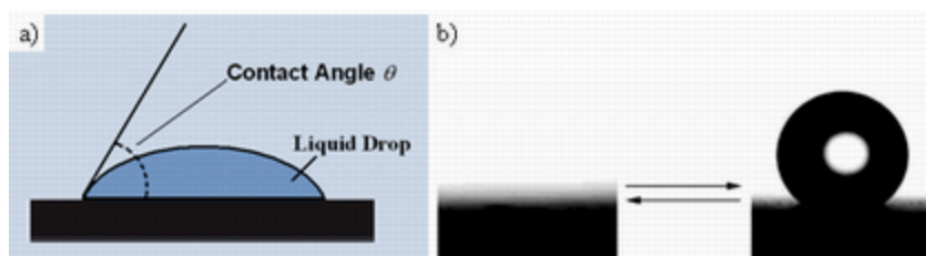
Figure 1: a) Contact angle measurement. b) Generic example of switching between superhydrophilic and superhydrophobic. 4
