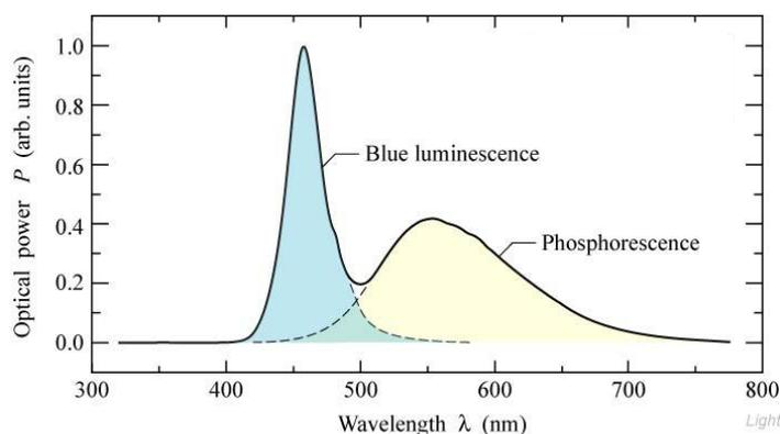
Figure 1. Emission spectrum of YAG:Ce-based white LED<sup>7</sup>
