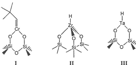
Sublimation of tetraneopentylchromium ( $\text{CrNp}_4$ ) onto a pyrogenic silica previously dehydrated at  $200^\circ\text{C}$  forms a product that consists of discrete  $\text{Cr}^{\text{IV}}$  dineopentyl units bound to the silica surface. When this product is heated at  $69^\circ\text{C}$  for 10 hours, one equivalent of neopentane is liberated and a silica-bound  $\text{Cr}^{\text{IV}}$  neopentylidene (I) is formed.
