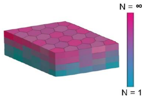
Figure 3: Vertical preferred orientation of perovskite films and random horizontal orientation 9
